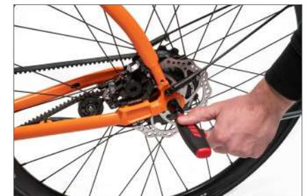
Before each ride, please check the correct tension of the **belt** or the **chain**; both need to be properly placed in location for the correct use.
