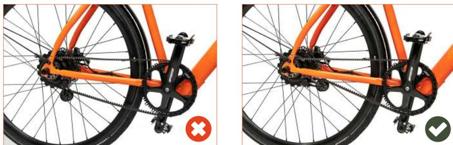
Verify that all bolts, fasteners of front and rear wheels, and kickstand (if any) are steady. Check that both **pedals** are properly tightened in the crank arms; if needed remove and reinstall the pedals, following the instructions in **Chapter 6**.
